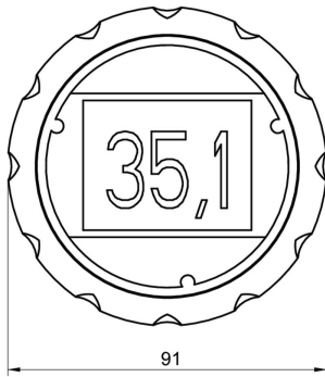
FlexHousing front view
