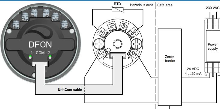
When fastening wires to the screw terminals a torque of 0.4Nm should be used.
