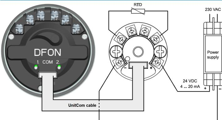
The FlexTop 22x2 has a plug for direct mounting to the DFON touch display from Baumer. The connection is established by using a UnitCom cable. Please contact Baumer for more information.
